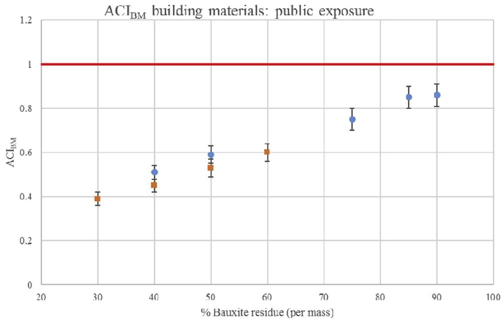
**Fig. 1.** Activity concentration index for building materials for different bauxite concrete mixtures with different % (by mass) of bauxite residue incorporation. Blue spheres represent the P-series, red squares represent C-series ( $k = 2$ ). Red line indicates threshold value of 1. (For interpretation of the references to colour in this figure legend, the reader is referred to the web version of this article.)
