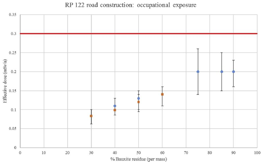
**Fig. 4.** Total effective dose for workers active in road construction in function of the different bauxite concrete mixtures with different % (by mass) of bauxite residue incorporation. Blue spheres represent the P-series, red squares represent the C-series. The red line indicates the dose criterion of 0.3 mSv/a proposed by RP122. (For interpretation of the references to colour in this figure legend, the reader is referred to the web version of this article.)
