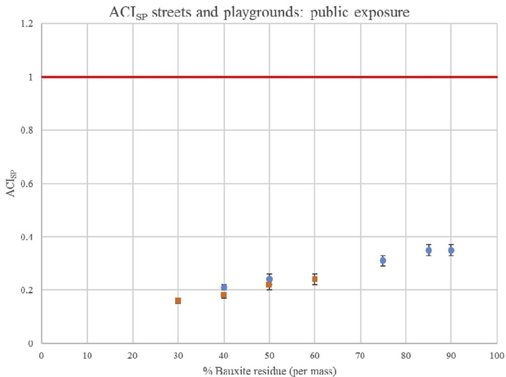
**Fig. 2.** Activity concentration index for streets and playgrounds for different bauxite concrete mixtures with different % (by mass) of bauxite residue incorporation. Blue spheres represent the P-series, red squares represent the C-series ( $k = 2$ ). Red line indicates threshold value of 1. (For interpretation of the references to colour in this figure legend, the reader is referred to the web version of this article.)
