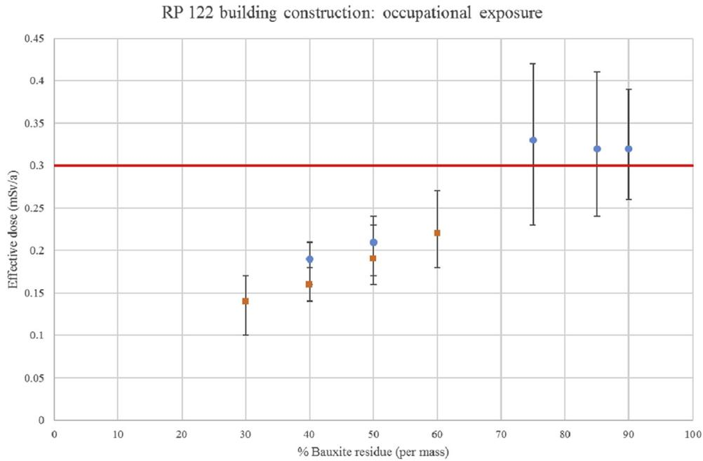
**Fig. 3.** Total effective dose for workers active in building construction in function of the different bauxite concrete mixtures with different % (by mass) of bauxite residue incorporation. Blue spheres represent P-series, red squares represent C-series. The red line indicates the dose criterion of 0.3 mSv/a proposed by RP122. (For interpretation of the references to colour in this figure legend, the reader is referred to the web version of this article.)
